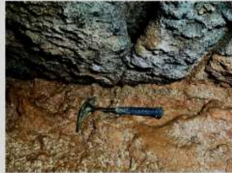
Fig.8. Stratigraphical unconformity boundary between 2 geological formations in T22 cave
