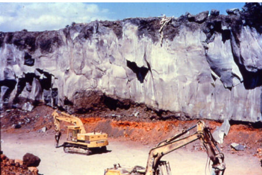
Fig. 1 - Quarry front displaying the cross flow section. The sequence of various layers and their different features can be noted: the upper dark-greyish layer is formed by scoriae. The intermediate layer is much more thick and light-greyish coloured and is formed by basaltic rock (« afficilàto »); it is currently exploited for hew lava stones production. The lower layer, of variable thickness, is made by « rifùsa » (re-molten), and down below the reddish « agghiàra » (gravel) layer can be detected (pict. by E. Lo Giudice)
